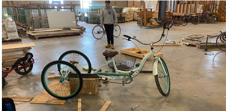
Extended back wheels of trike for longer cargo component
