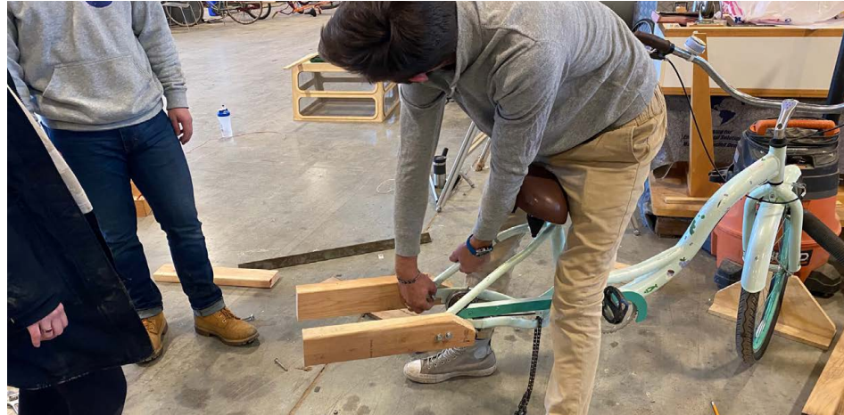
Using plywood as a testing material to determine distance and strength of connection
