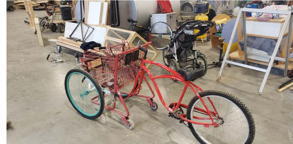
Attached the grocery cart handle to the head of the bike.
