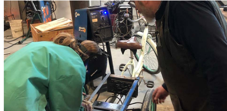
Welding of flat base component for the attachment of various cargo components
