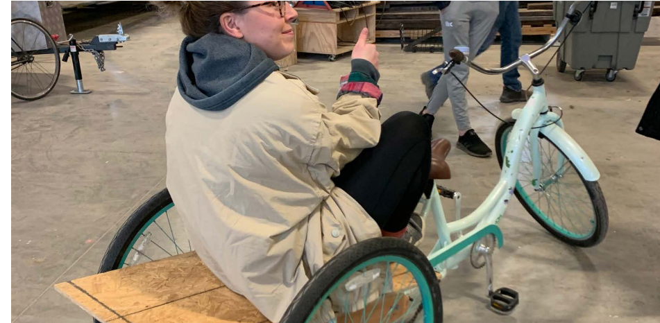
Testing load capacity for back load component and attachability of flat base
