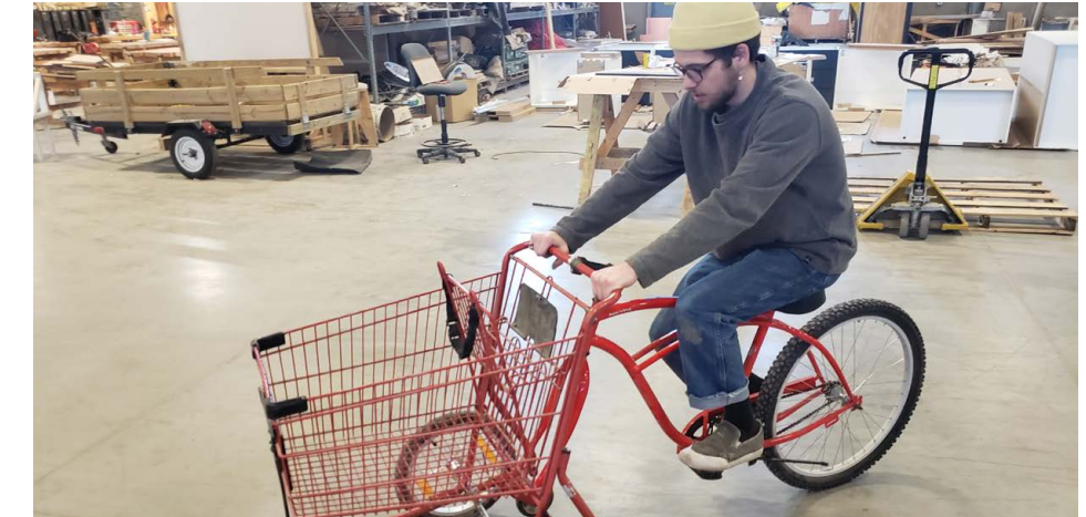
Attached burley wheels to solid rod axle.
